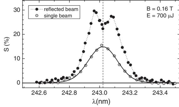
FIG. 1. Line shapes measured with a laser bandwidth of  $\sim 100$  GHz with and without the retro-reflected beam. The solid black line is a Gaussian fit that yields a centroid of  $243.0208 \pm 0.0016$  nm and a FWHM of  $0.226 \pm 0.005$  nm. The dotted line in the reflected beam data is a simple spline fit. The dashed vertical line is at  $243.0218$  nm, (to be compared to measurements from Fig. 3).
