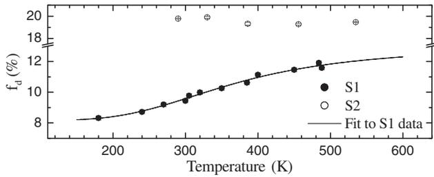
FIG. 2.  $f_d$  as a function of temperature for  $S1$  (filled circles) and  $S2$  (open circles) taken at the low beam density. The  $S2$  data were taken using a reduced magnetic field of 0.15 T to minimize the effect of radiation damage, which leads to an increase in  $f_d$ . A fit was made to the  $S1$  data using the procedure described in the text.
