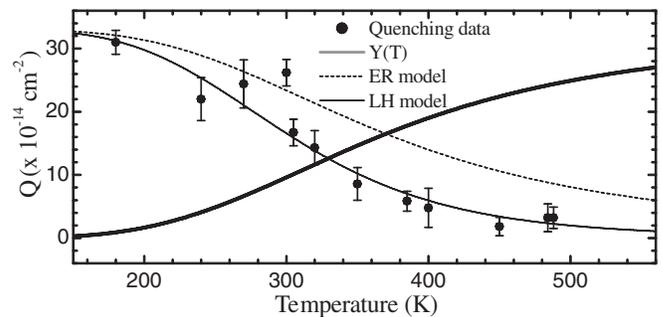
FIG. 4. The quenching in sample  $S1$  as a function of the temperature. The thermal positronium yield  $Y(T)$  was obtained from a fit to the data shown in Fig. 3 and has been scaled to fit the amplitude of the quenching signal. The expected ER and LH model curves are plotted as described in the text.
