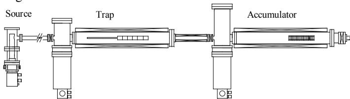
**FIGURE 1.** A schematic layout of the positron source, accumulator and trap. This system is essentially the same as a standard Surko trap except that the final accumulation region is in a separate vacuum system, which allows us to obtain long lifetimes since the pressure is reduced.
