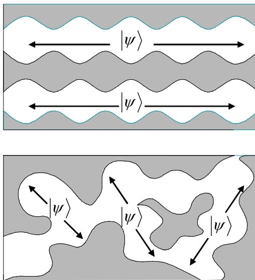
**FIGURE 4.** Two separate targets with interconnected pores were used. The top panel shows a target in which the pores are aligned into 1-dimensional channels, which means that there is a continuum of accessible eigenstates for Ps atoms contained therein. The bottom panel is a representation of a sample in which the pores are interconnected but randomly orientated; here, at low energies, only discrete eigenstates are accessible.
