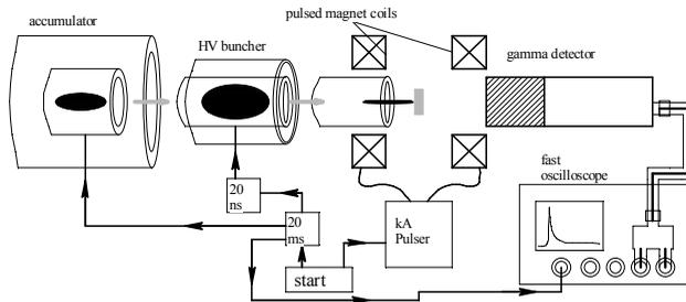
**FIGURE 2.** The firing sequence for data acquisition using SSPALS. As soon as the positron accumulation phase is complete and all required plasma manipulations have been performed a start signal begins the sequence. Because of its inductance it takes around 20 ms for the magnet to come on, and the HV buncher must be delayed by around 20 ns to account for the transit time of the positron plasma from the accumulator.
