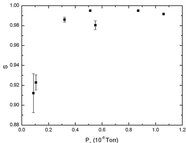
Fig. 2. Sticking coefficient  $S$  of  $N_2$  gas on a 12 K surface as a function of  $N_2$  gas pressure  $P_1$ .
