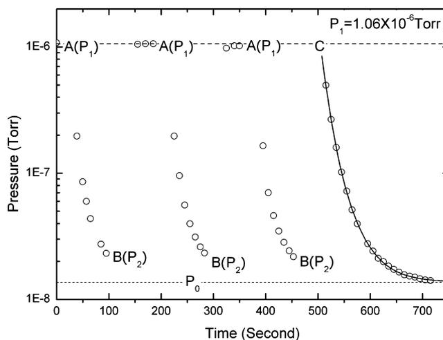
Fig. 1. Typical measurement of pressure as a function of time. At A, the nozzle was moved to the front of the cold finger, and at B, the nozzle was moved to the outside of the shield. At C, the leak valve is being closed.
