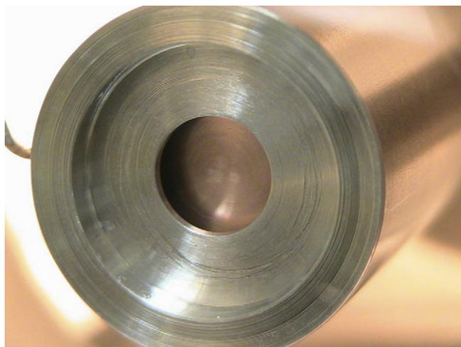
Fig. 3. Three white nitrogen spots in the center and the ring fringe pattern. The scale size is given by the 9 mm opening in the cold shield in front of the face of the Cu cold finger. The condensation spots are about 1 mm in diameter, which is close to the size of the opening in the gas deposition nozzle.
