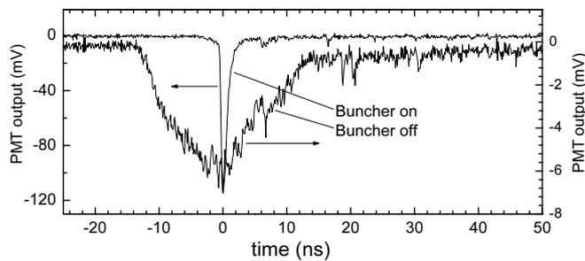
**Fig. 2** Positron beam time compression with and without the buncher.
