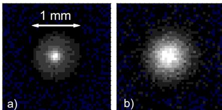
**Fig. 3** Beam profiles at high (a) and low (b) density.
