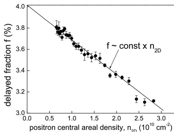
**Fig. 5** The reduction in the amount of long lived Ps is a linear function of the areal density.
