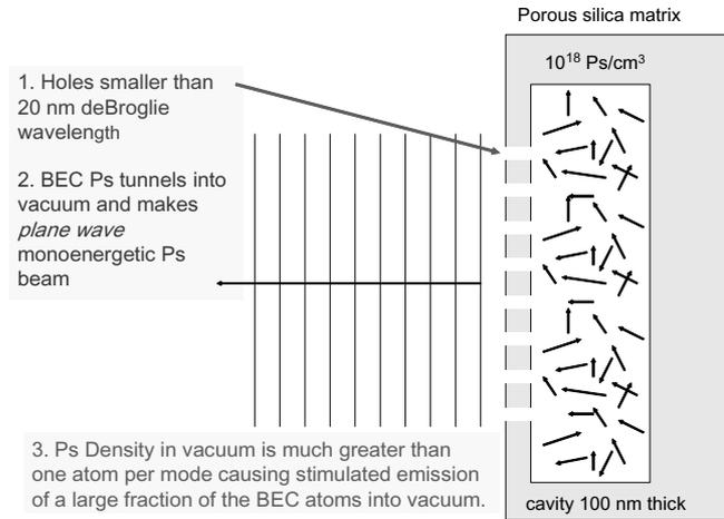
**Fig. 10** A Ps atom laser may be produced via a Ps BEC.
