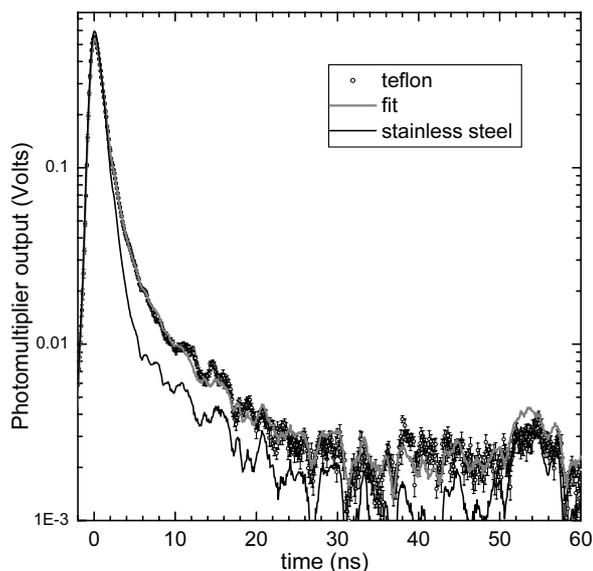
**Fig. 6** A single shot lifetime spectrum with Teflon and a stainless steel target, the latter used as a system response function which was then used in the fitting procedure.
