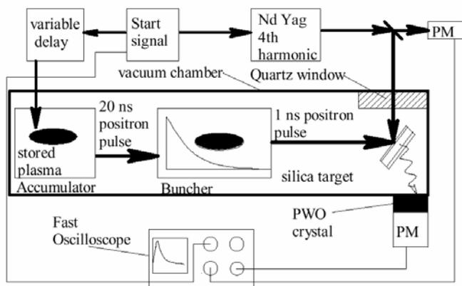
**Fig. 7** A schematic of the layout of the laser timing and gamma ray detection system.
