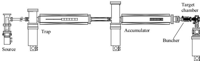
**Fig. 1** A schematic of the positron source, trap, accumulator and target chamber.
