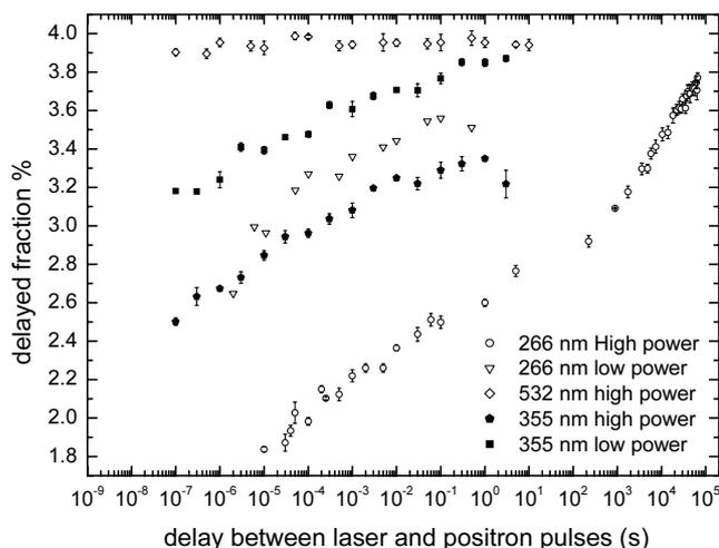
**Fig. 8** The delayed fraction as a function of time for various laser powers and wavelengths. Low power refers to  $\sim 3$  mJ/pulse, and high power  $\sim 10$  mJ/pulse.
