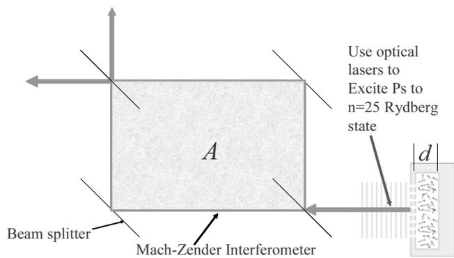
**Fig. 11** A Ps atom beam laser could be used in a Mach-Zender interferometer to measure the Ps gravitational interaction.
