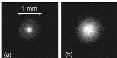
FIG. 12. The effect of the pulsed magnet on the beam compression. Image (a) is a fully compressed plasma with an areal density of around  $3 \times 10^{10} \text{ cm}^{-2}$  while (b) has been allowed to expand for 3 s before being ejected from the accumulator, producing a beam with an areal density of  $4.9 \times 10^9 \text{ cm}^{-2}$ .
