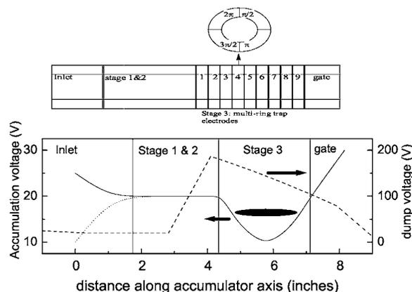
FIG. 5. Above: the accumulator electrode structure. The phases of the rf signal are indicated in the split ring. Below: the axial potential profiles for storing (solid line) and dumping (short dashed line) positron plasmas. The dotted line indicates the momentary ( $\sim 100$  ns) opening of the inlet to admit a pulse from the trap.
