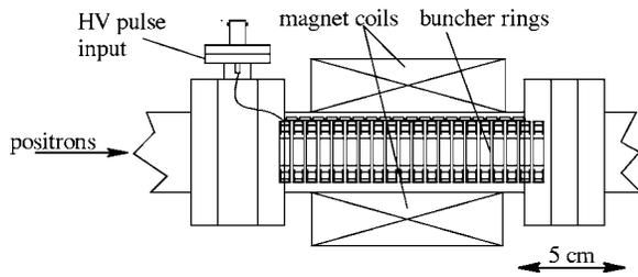
FIG. 8. The buncher layout. The bunching potential gradient was established by a string of resistors connecting neighboring accelerator rings with a total resistance of 50  $\Omega$ . Each resistor was formed from a short length of 100  $\Omega$ /ft resistance wire spot welded between two rings.
