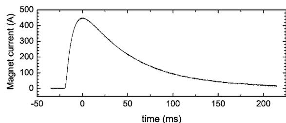
FIG. 11. The pulsed magnet current. The arrival of the positron pulse is tuned to coincide with the maximum magnetic field to maximize compression.
