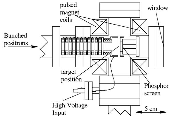
FIG. 10. The layout of the accelerator rings and the phosphor screen used to image the beam. The accelerator rings are interconnected in pairs by 1 M $\Omega$  KDI Pyrofilm vacuum compatible resistors and allow the beam to be accelerated up to 10 kV without the use of grids. The accelerator voltage is applied only for a short time to prevent overheating the resistors.
