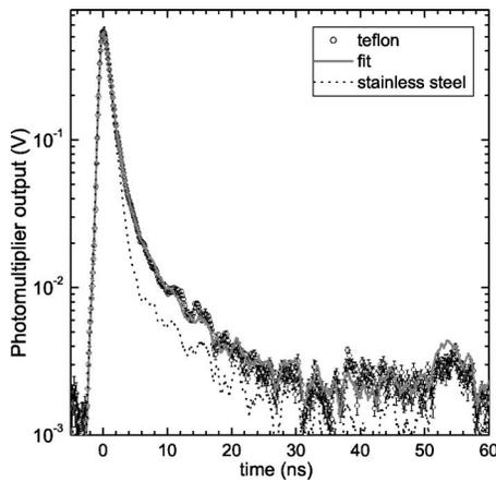
FIG. 14. Positronium lifetime spectrum in a Teflon sample using a  $\text{PbF}_2$  crystal attached to an R2287U photomultiplier. The timing resolution is 1.55 ns FWHM and the pulse width is  $<1$  ns. The small amplitude fine scale structure is due to small cable reflections. The feature at about 54 ns appears to be an ion after pulse similar to that observed in the XP2020 PMT.
