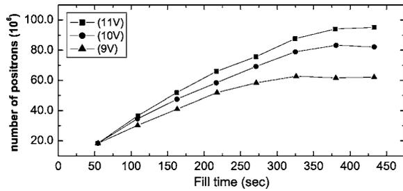
FIG. 6. A positron stacking curve in which the effect of lowering the well depth (indicated in the legend) increases the maximum number of positrons that can be stored.
