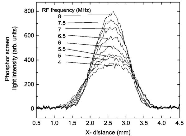
FIG. 7. Radial profiles of the positron plasma as a function of the applied rotating wall frequency, as measured by dumping the plasma onto phosphor screen biased to  $-5$  kV and imaging it using a CCD camera. The plasmas shown in this figure contained around  $2 \times 10^7$  positrons.
