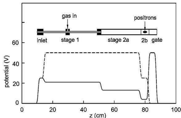
FIG. 2. Above: scaled drawing of the trap electrode structure. Below: the axial potential profiles for trapping (solid line) and releasing (“dumping”) positrons (dashed line).
