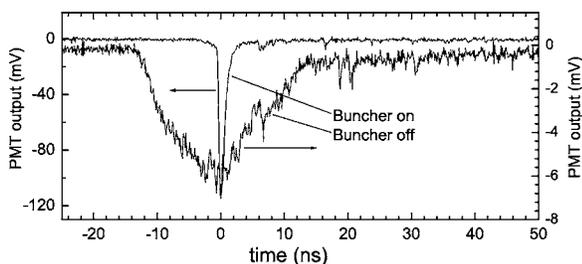
FIG. 9. The time width of the pulse with and without the buncher. The  $\sim 20$  ns FWHM pulse emitted from the accumulator is compressed into a subnanosecond pulse with practically no loss of particles. The “buncher off” trace has been slightly displaced vertically for clarity.
