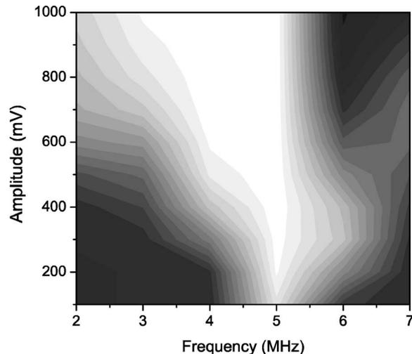
FIG. 4. Amplitude-frequency scan of trapping efficiency for the rf signal applied to the rotating wall electrode in the trap. The color shade indicates the efficiency, with white corresponding to the maximum value of approximately 20%.
