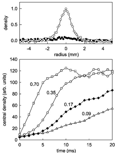
FIG. 3. Above: radial profiles of positrons in the trapping section. (●) without rf applied; (○) with rf applied. Below: central density of the positron cloud as a function of time for various values of applied rf signal amplitude, shown in the figure in volts. The rf was switched on at  $t=0$ .
