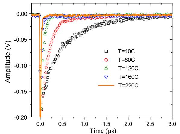
Fig. 4. Some anode traces for various temperatures of the  $\text{BaF}_2$  scintillator. The original waveforms have been interpolated into 200 points. The  $t = 0$  time coincides with the peak of the prompt. To better visualize the slow decay, the traces have been truncated at amplitudes  $V = -0.2\ \text{V}$ .
