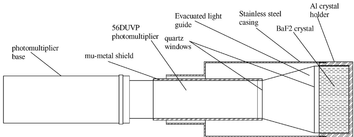
Fig. 2. The design of the BaF<sub>2</sub>-PM system adopted in this experiment. Details are described in the text.
