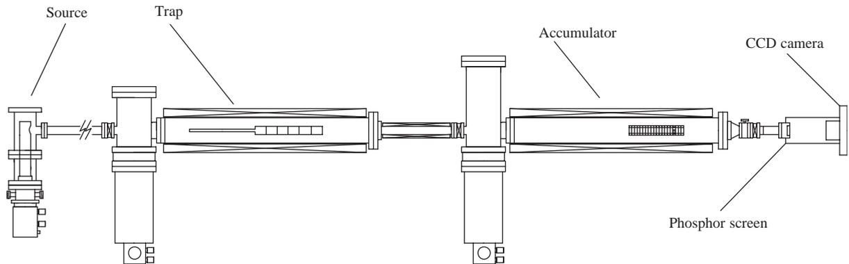
Fig. 1. The layout of the positron accumulator system. A DC positron beam of  $8 \times 10^6/s$  is generated by the solid neon moderator in the source. From this the trap section created pulses containing approximately 250,000 positrons and delivers them to the accumulator at 4 Hz. The accumulator is capable of storing  $1 \times 10^8$  positrons and can deliver pulses with a spread of approximately 10 ns.
